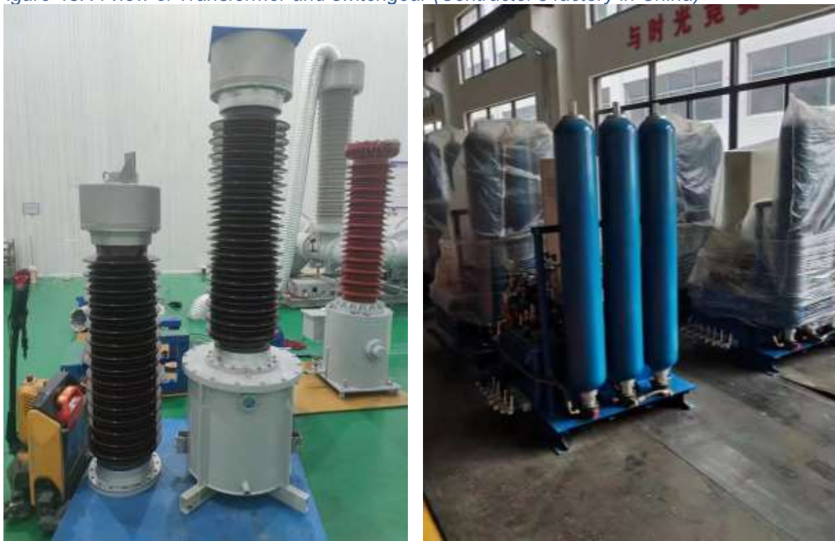
Figure 47: Instrument transformer being factory tested (left) and Lot 7 Hydraulic system of MIV (right) at Contractor's factory in China
