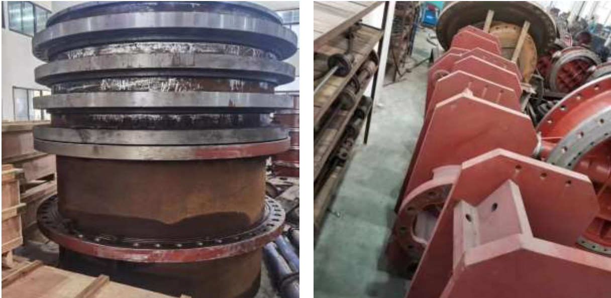
Figure 44: MIV being manufactured at Contractor’s factory in China
