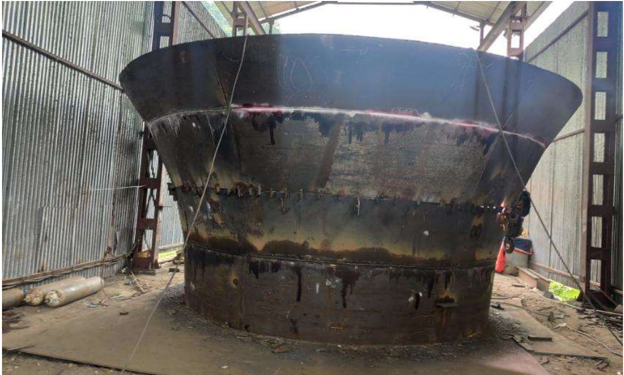
Figure 39: Fabrication of bellmouth
