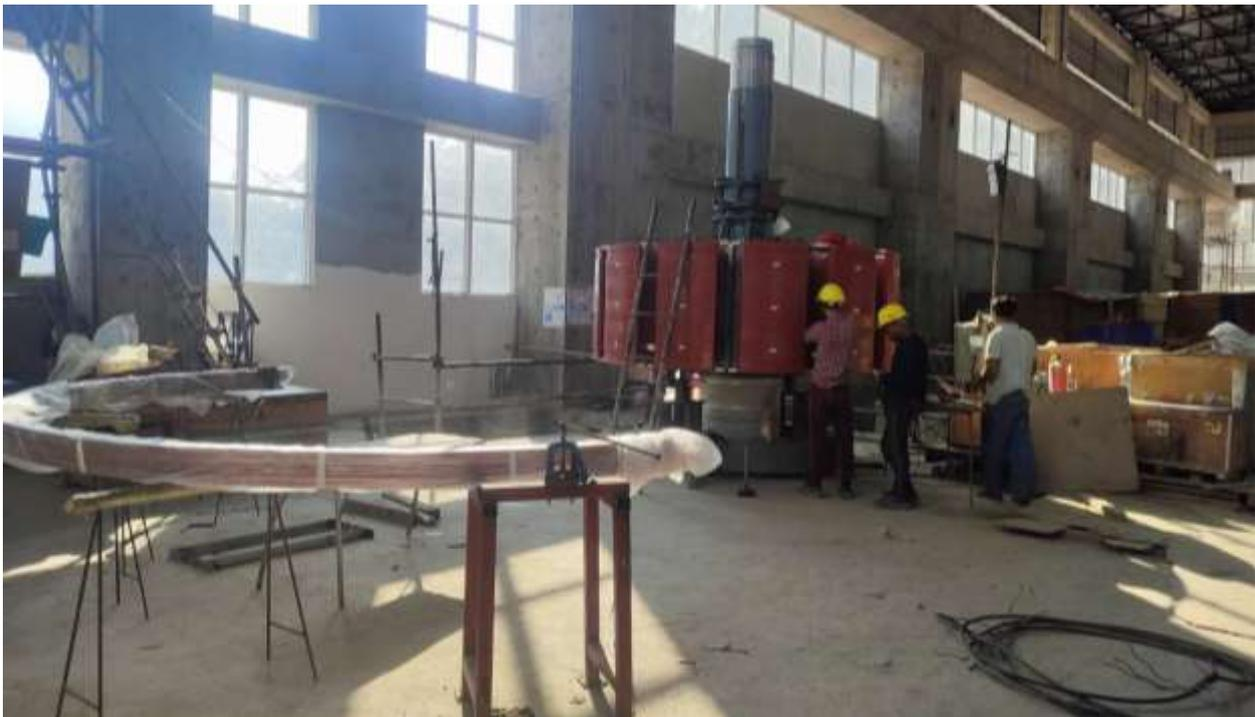
Figure 2-48: Final assembly of magnetic poles for rotor
