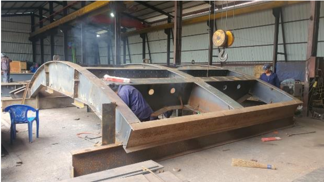
Figure 2-37: Fabrication of radial gates
