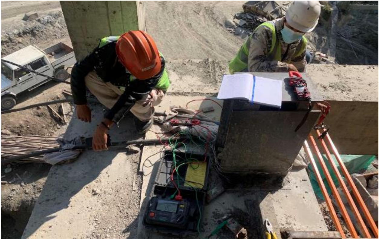
Figure 2-45: Insulation Resistance of EOT's busbar
