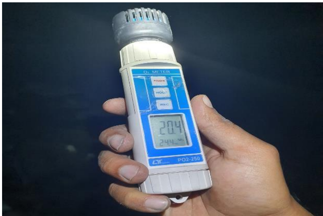
Figure 58: Monitoring of quality of air inside Tunnel on daily basis
