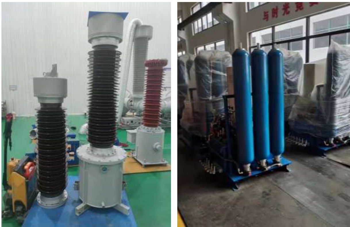
Figure 44: Instrument transformer being factory tested (left) and Lot 7 Hydraulic system of MIV (right) at Contractor's factory in China
