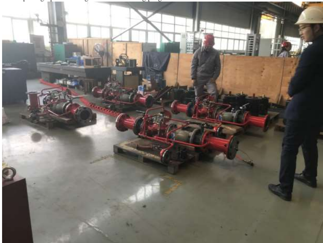
Figure 2-49: Fire fighting valve getting ready for testing
