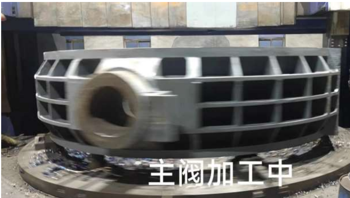
Figure 2-53: PPV body being machined
