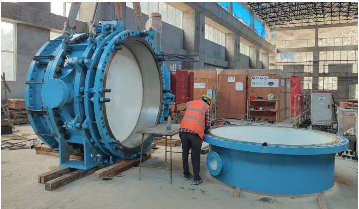
Figure 2-75: MIV assembled at service bay
