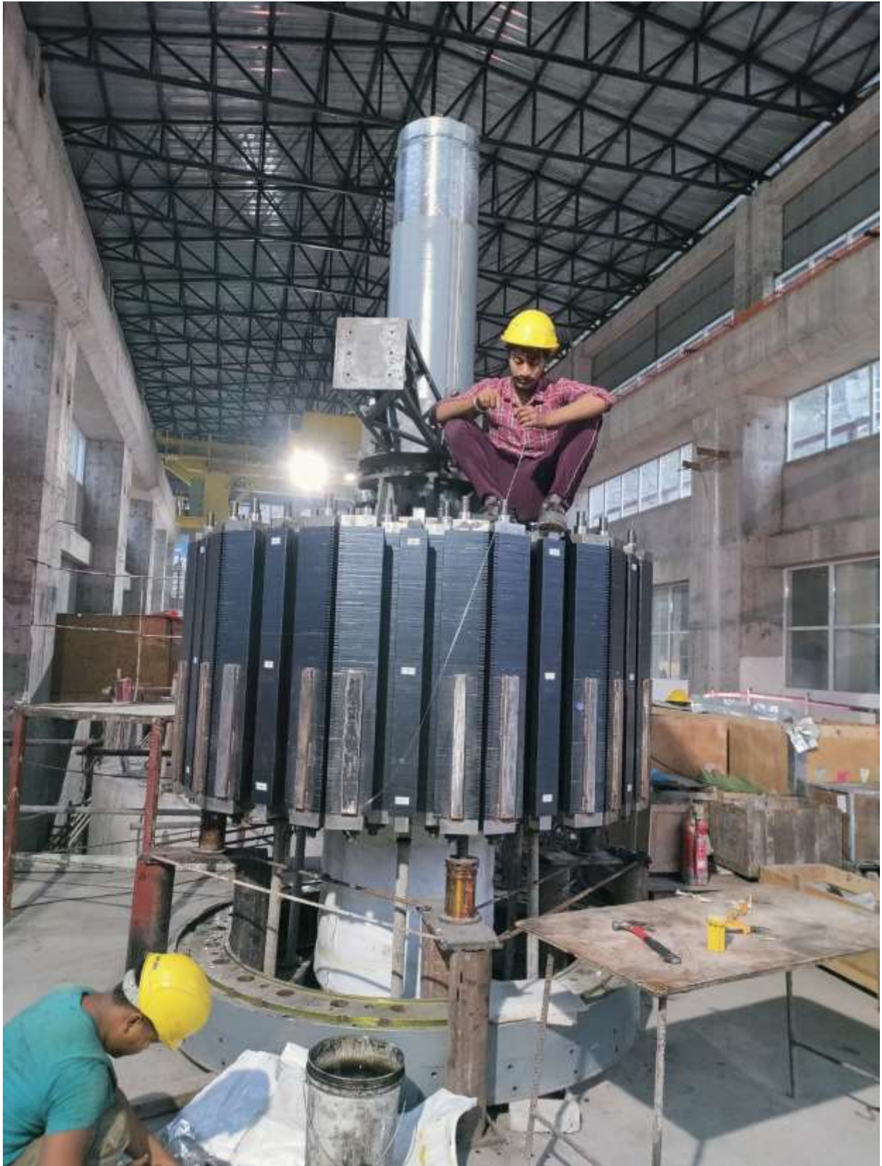
Figure 2-61: Magnetic yoke assembly of rotor
