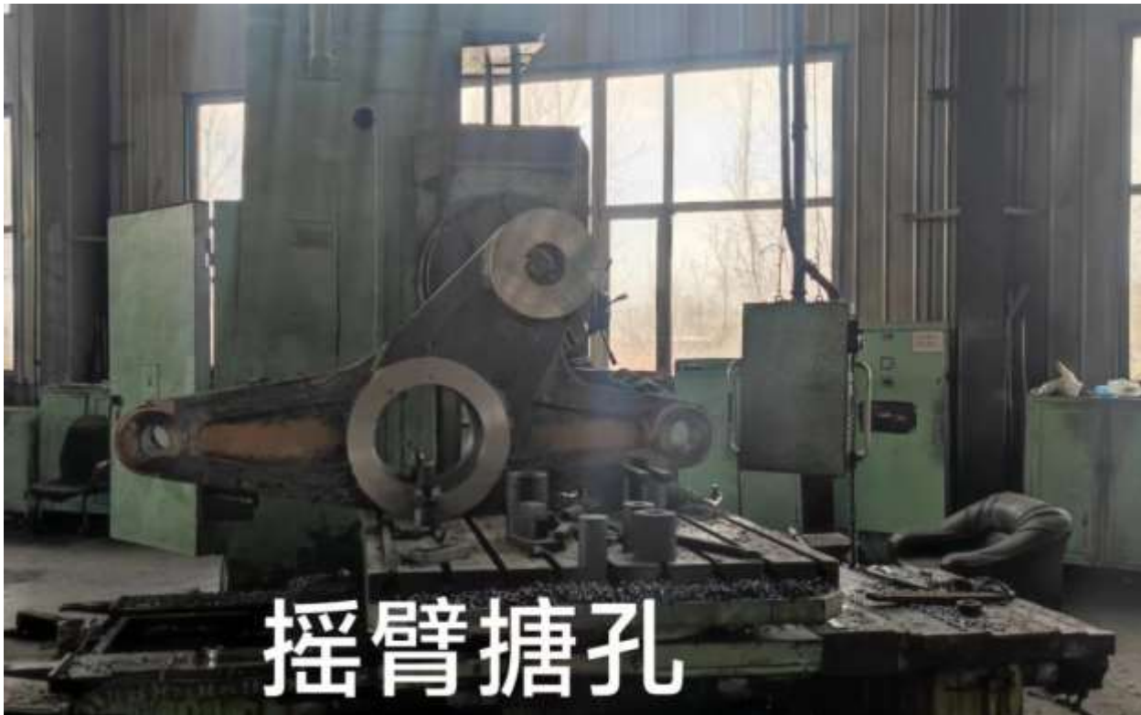
Figure 2-55: PPV swing body being machined
