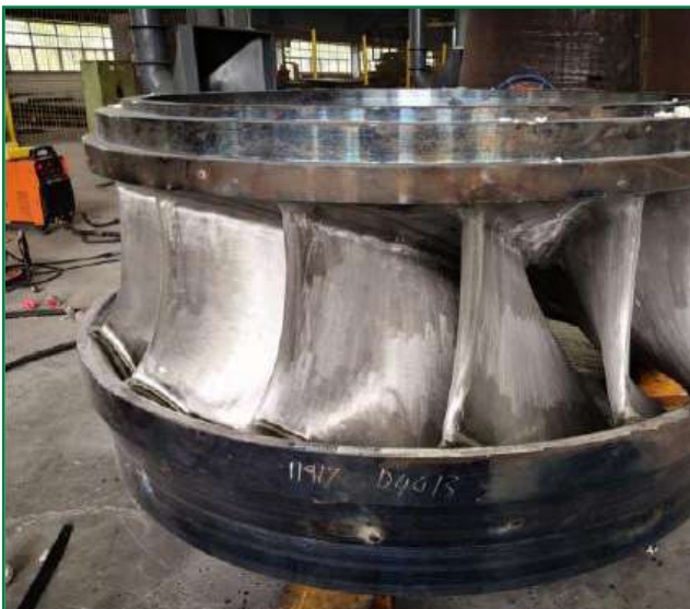
Fabrication of runner (left) and lamination works of rotor (right)
