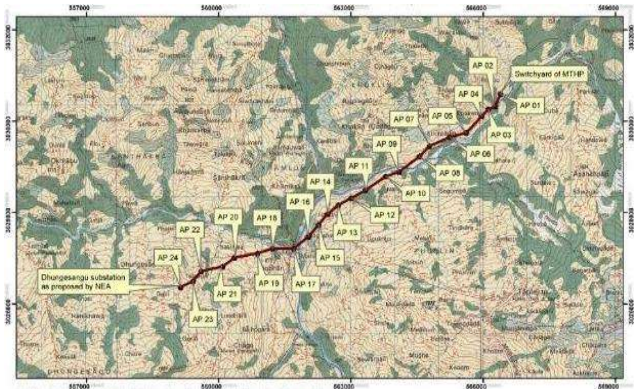
Figure 2-53: Transmission line route map
