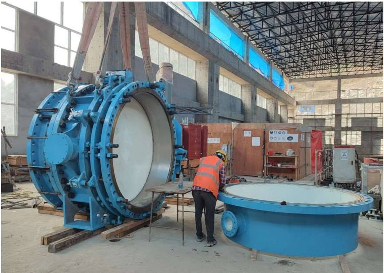
Figure 2-51: Unit 2 MIV assembled at Service bay
