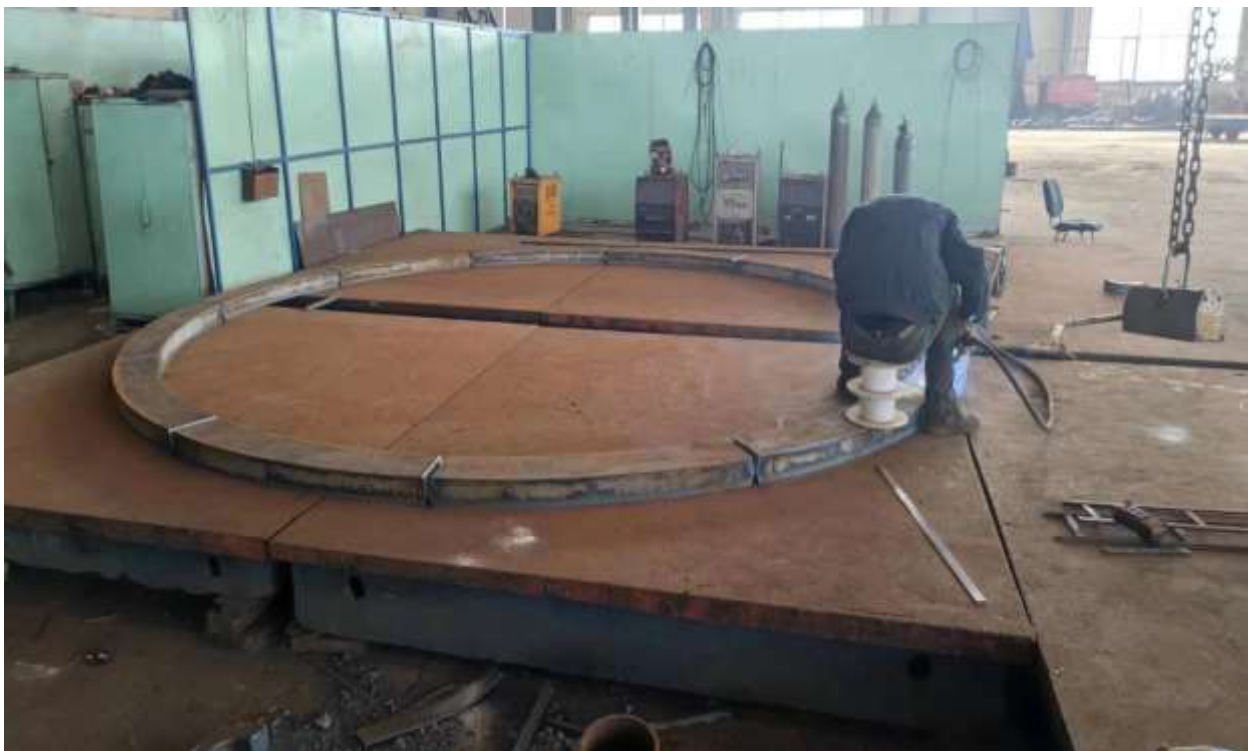
Figure 38: Flange being manufactured at the Contractor's Factory in China
