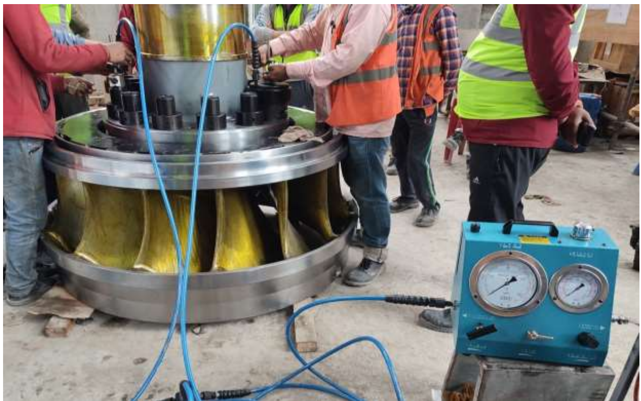
Figure 2-61: Assembly of runner with main shaft
