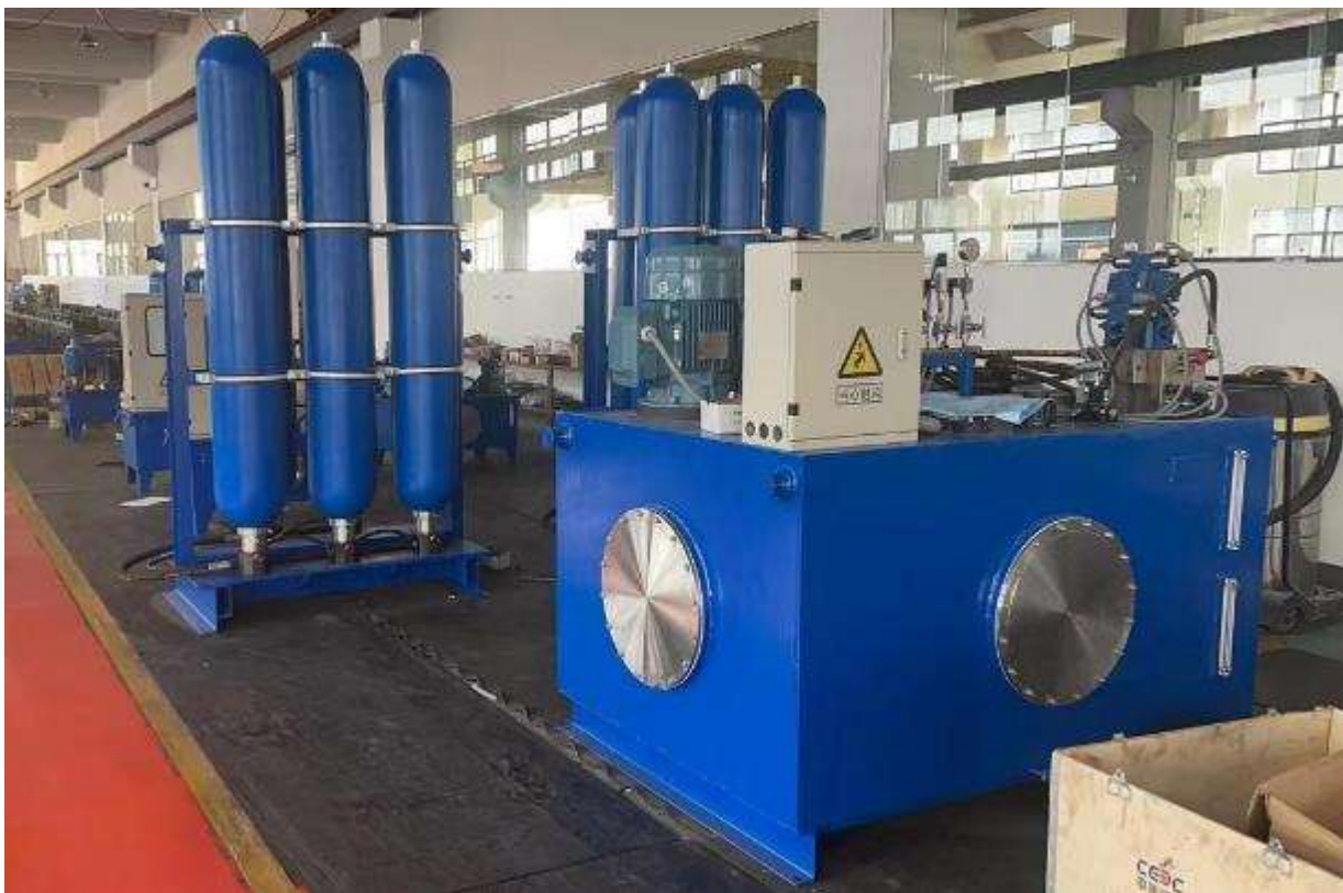
Figure 2-47: PPV hydraulic system ready for dispatch
