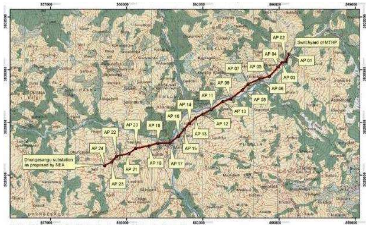
Figure 2-75: Transmission line route map
