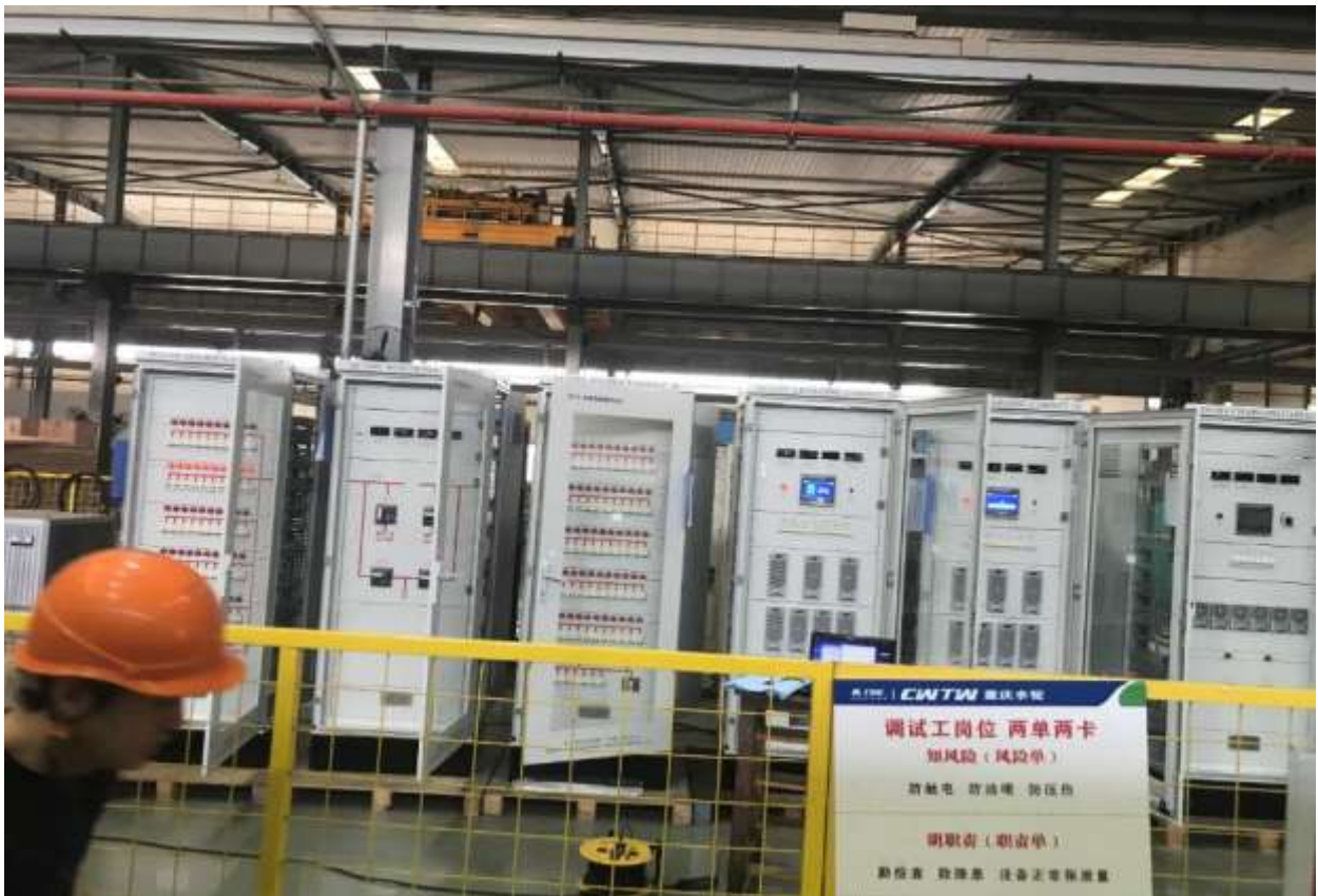
Figure 2-46: DC panels are ready to be dispatched at CWTW factory, China
