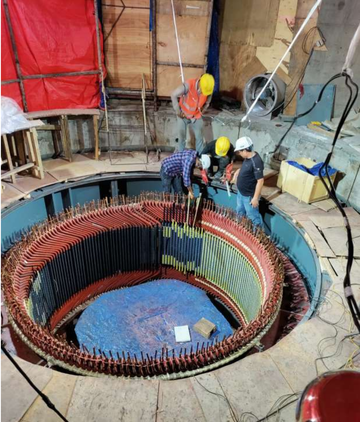
Figure 2-54: High voltage AC test of stator coils
