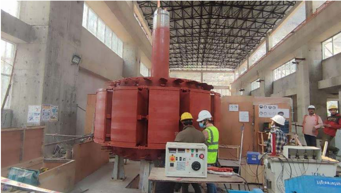
Figure 2-56: A.C. withstand voltage test of rotor winding
