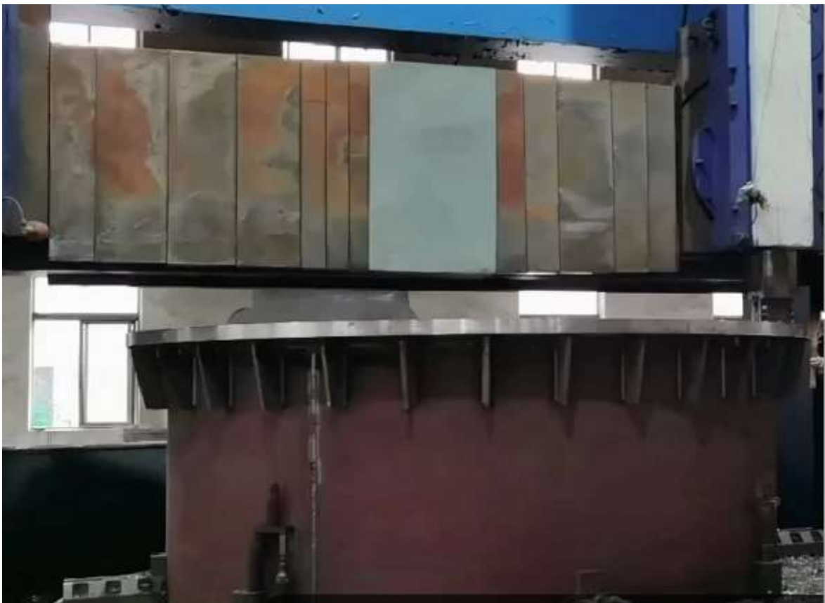
Figure 2-50: Machining works of connecting pipe in China
