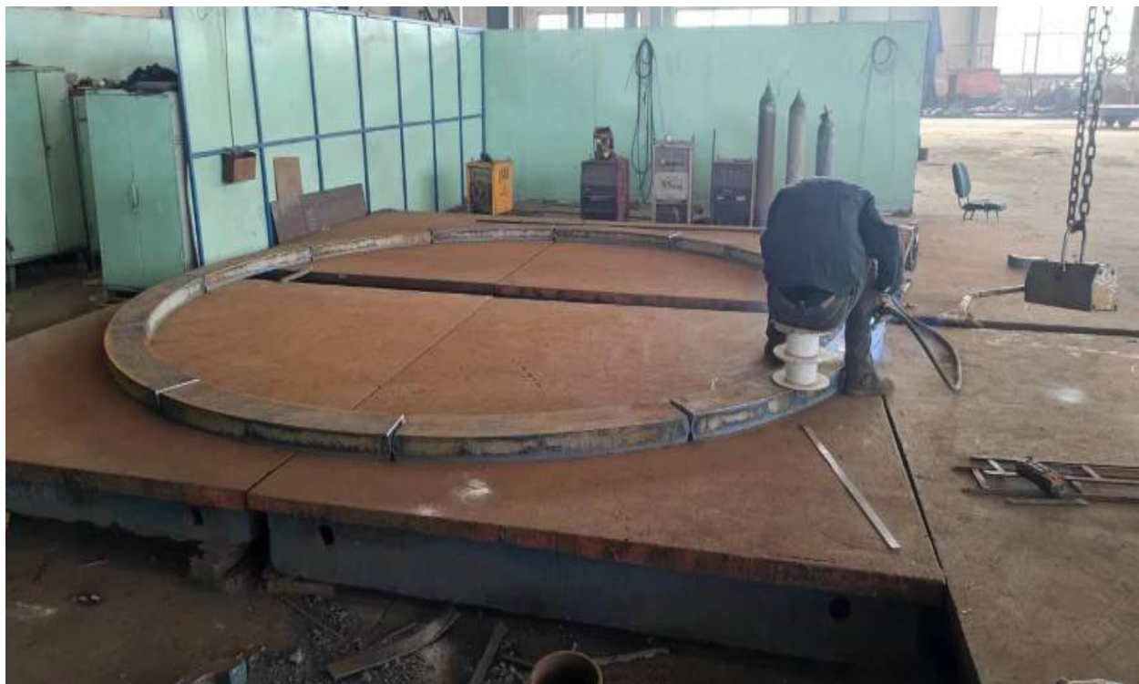
Figure 2-30: Flange being manufactured at the Contractor's Factory in China
