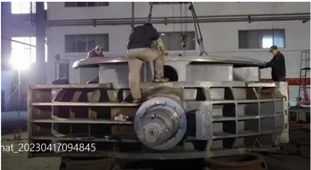
Figure 2-28: PPV disc being assembled with PPV body
