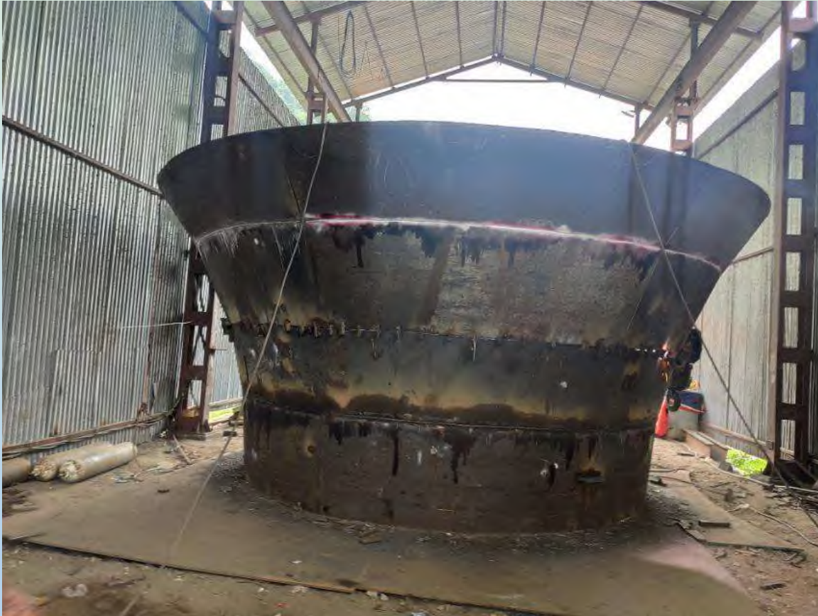
Fabrication of bell mouth for approach pipe
