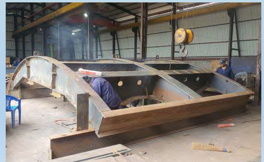
Fabrication of radial gates at Pokhara workshop
