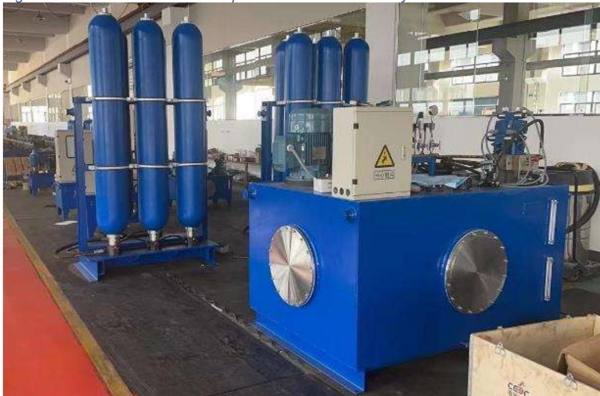
Figure 2-50: PPV hydraulic system ready for dispatch
