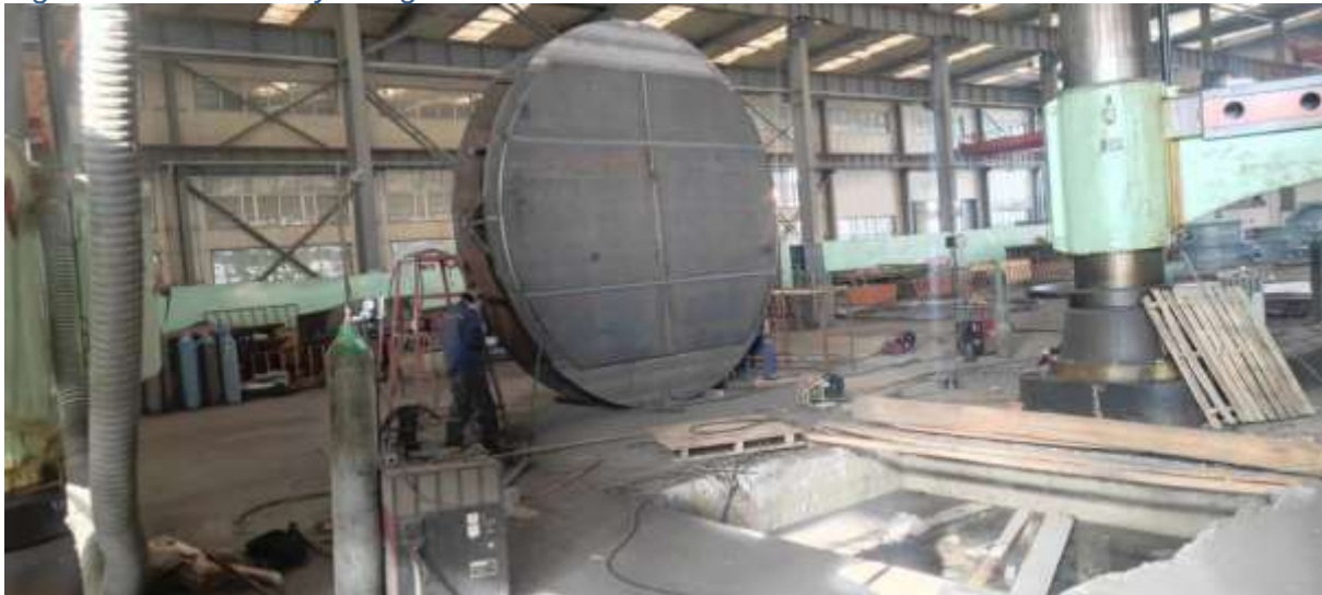
Figure 2-52: PPV disc being welded
