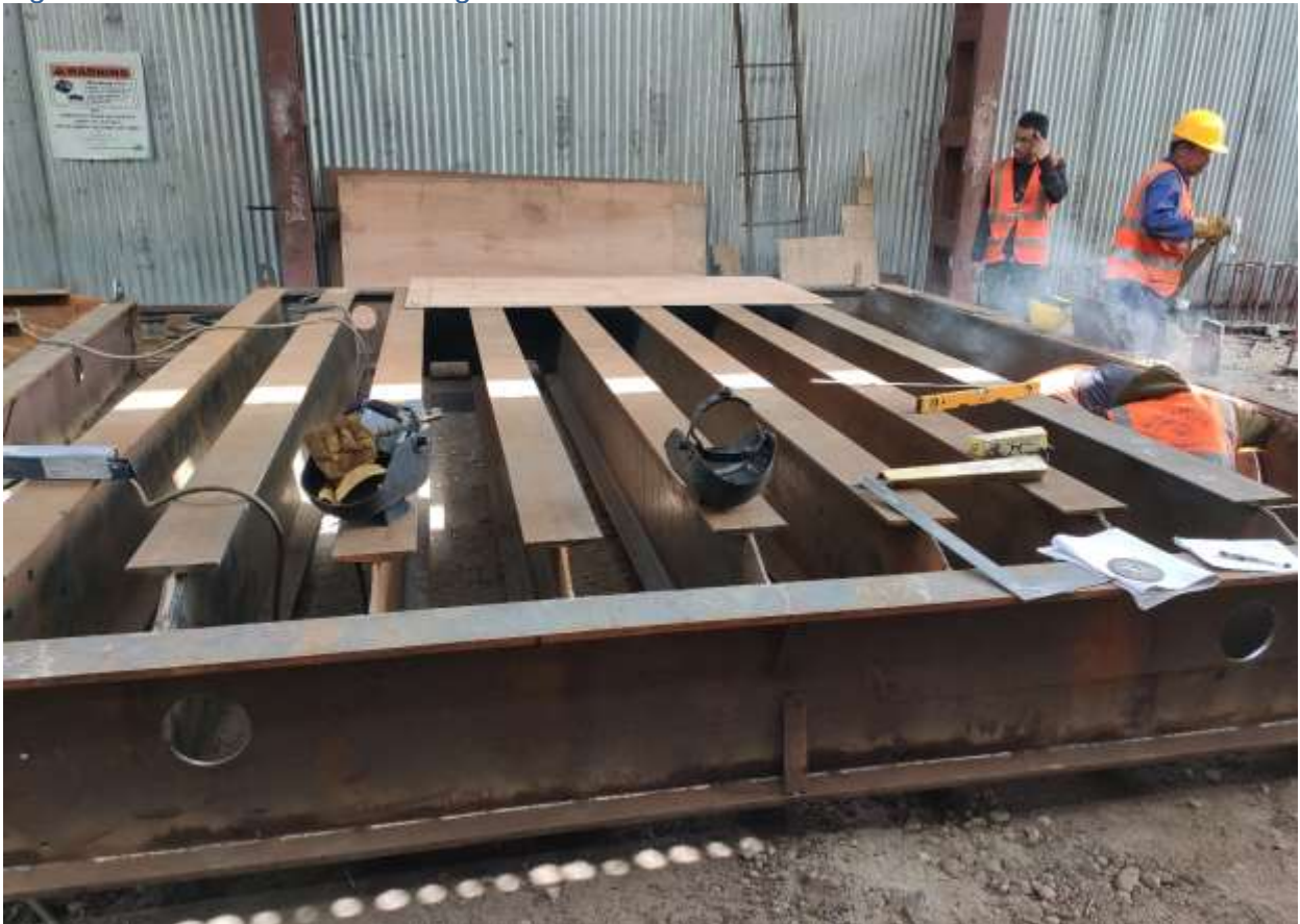
Figure 2-43: Fabrication of intake gate
