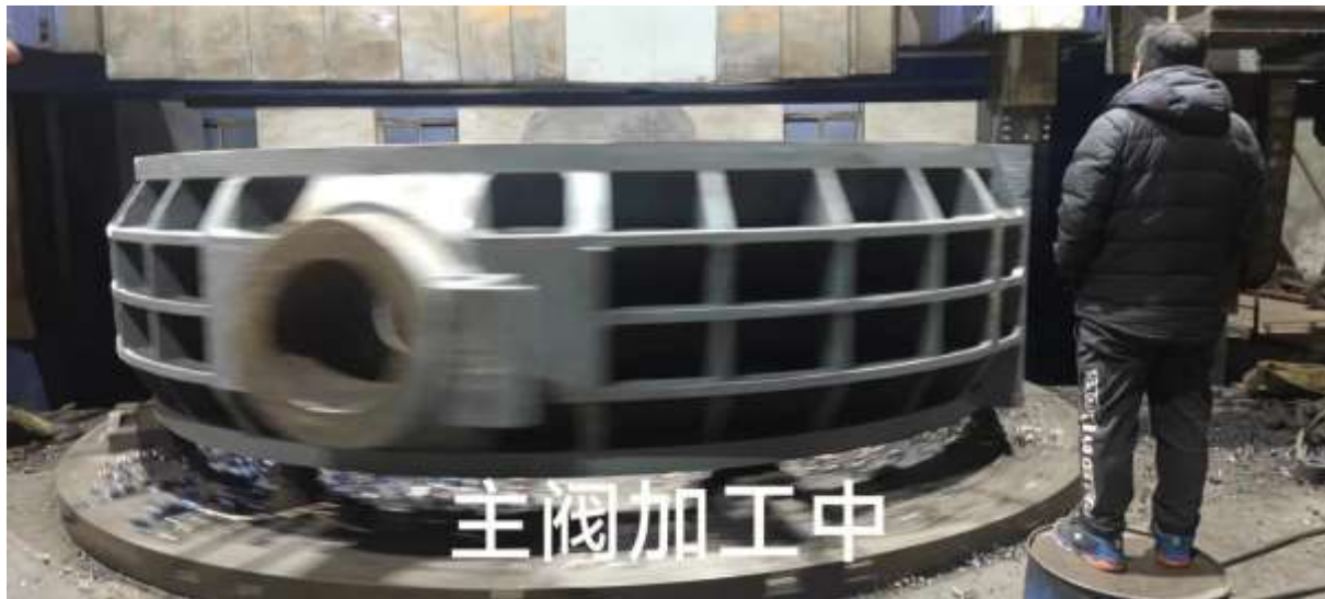
Figure 2-51: PPV body being machined
