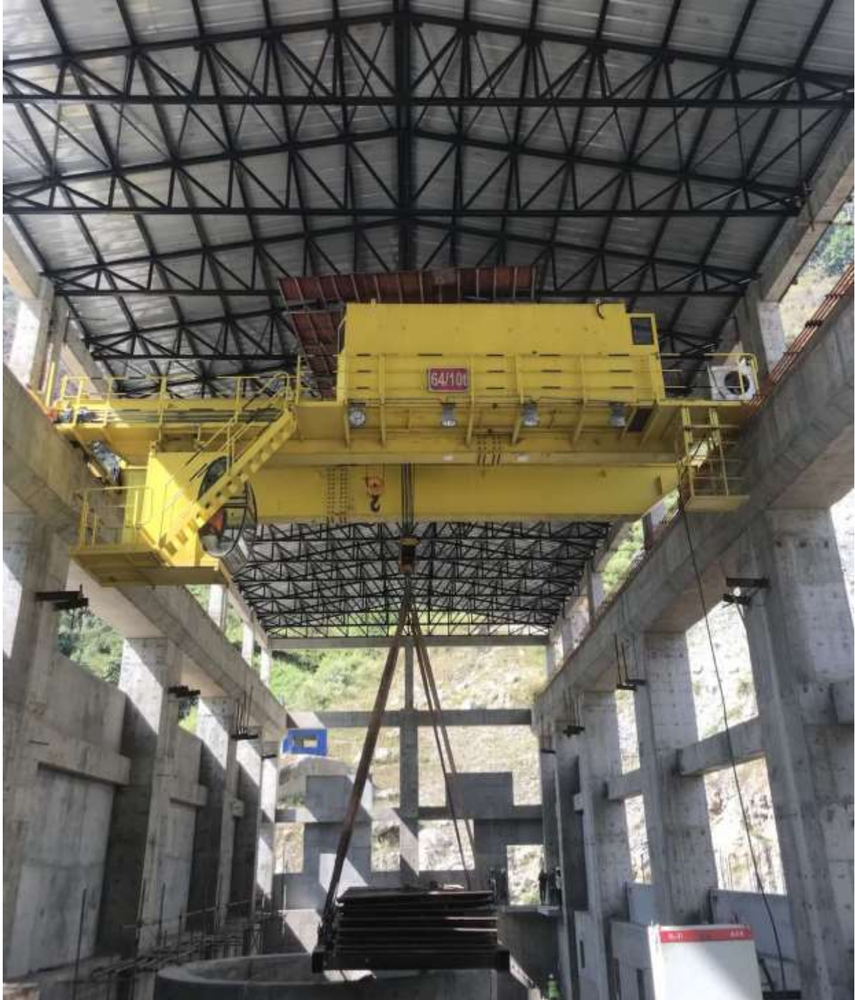
Figure 2-56: Load test of EOT lifting 66 ton and travelling across unit 2
