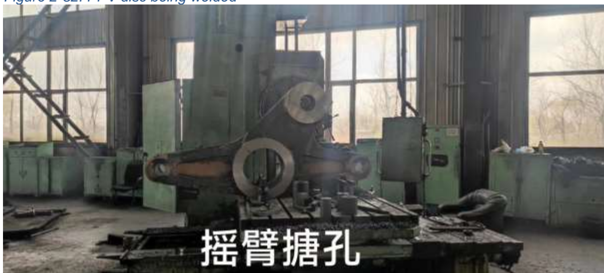
Figure 2-53: PPV swing body being machined
