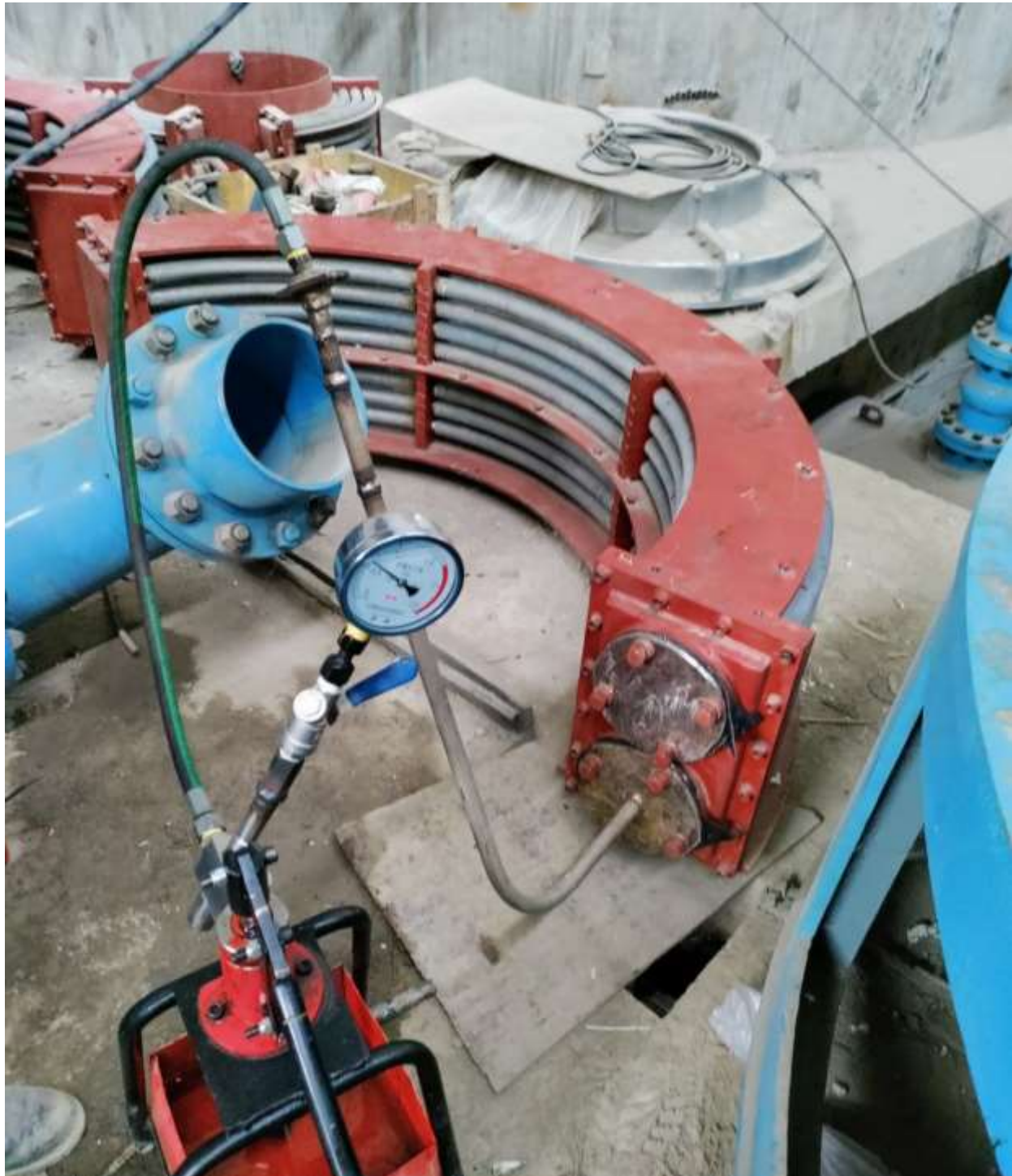
Figure 2-52: Pressure test of upper bracket bearings oil cooler
