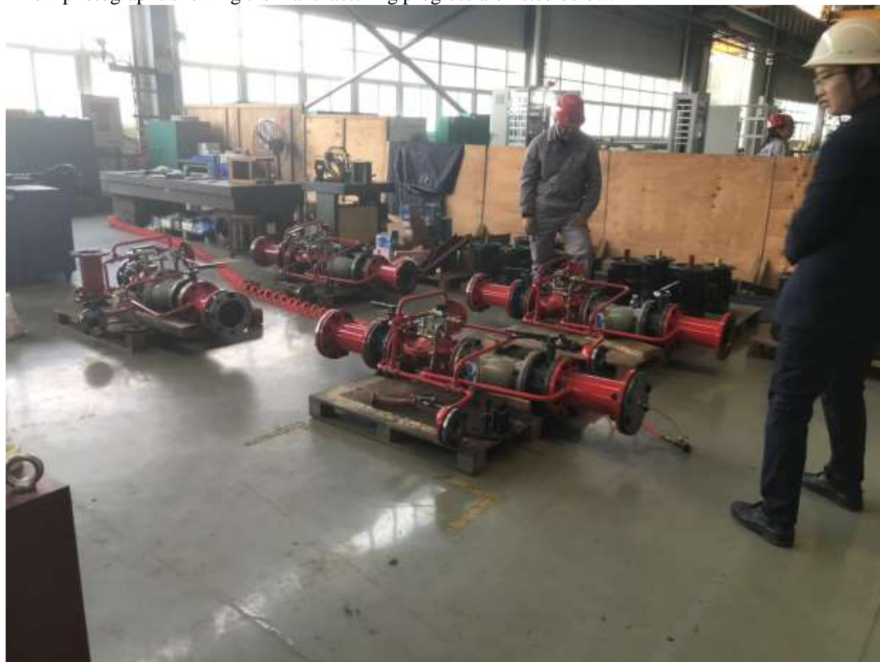
Figure 2-40: Fire fighting valve getting ready for testing
