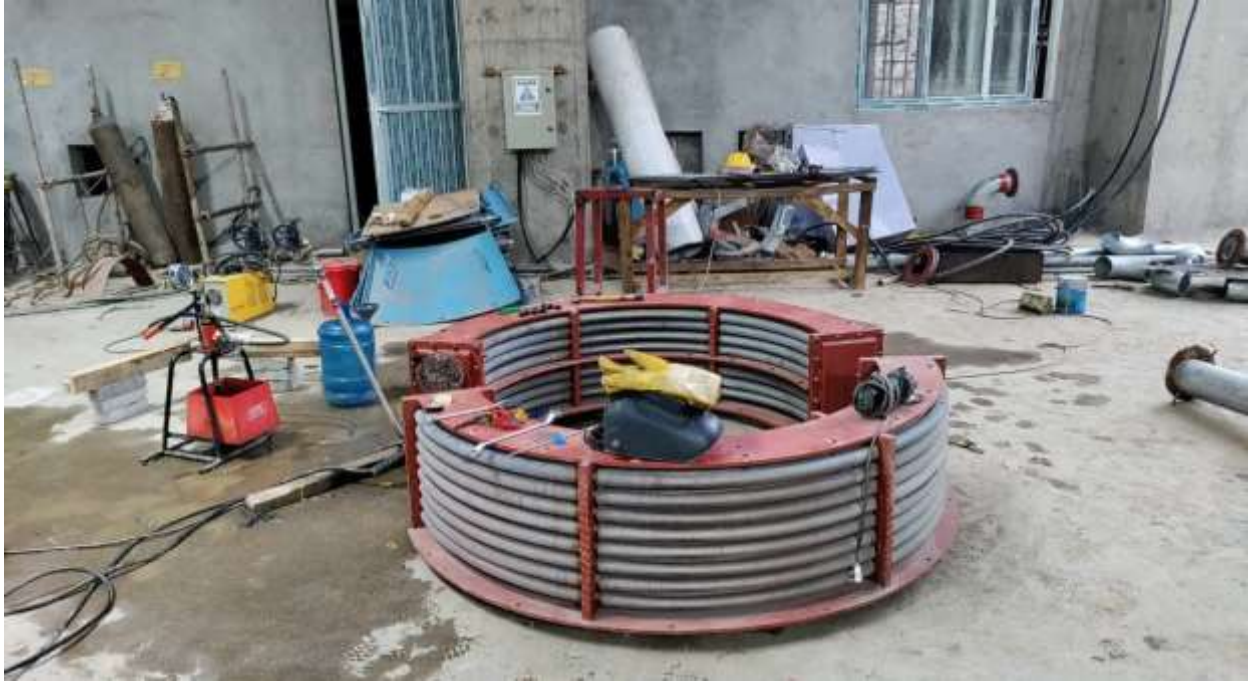
Figure 2-48: Pressure test of upper bracket bearings oil cooler
