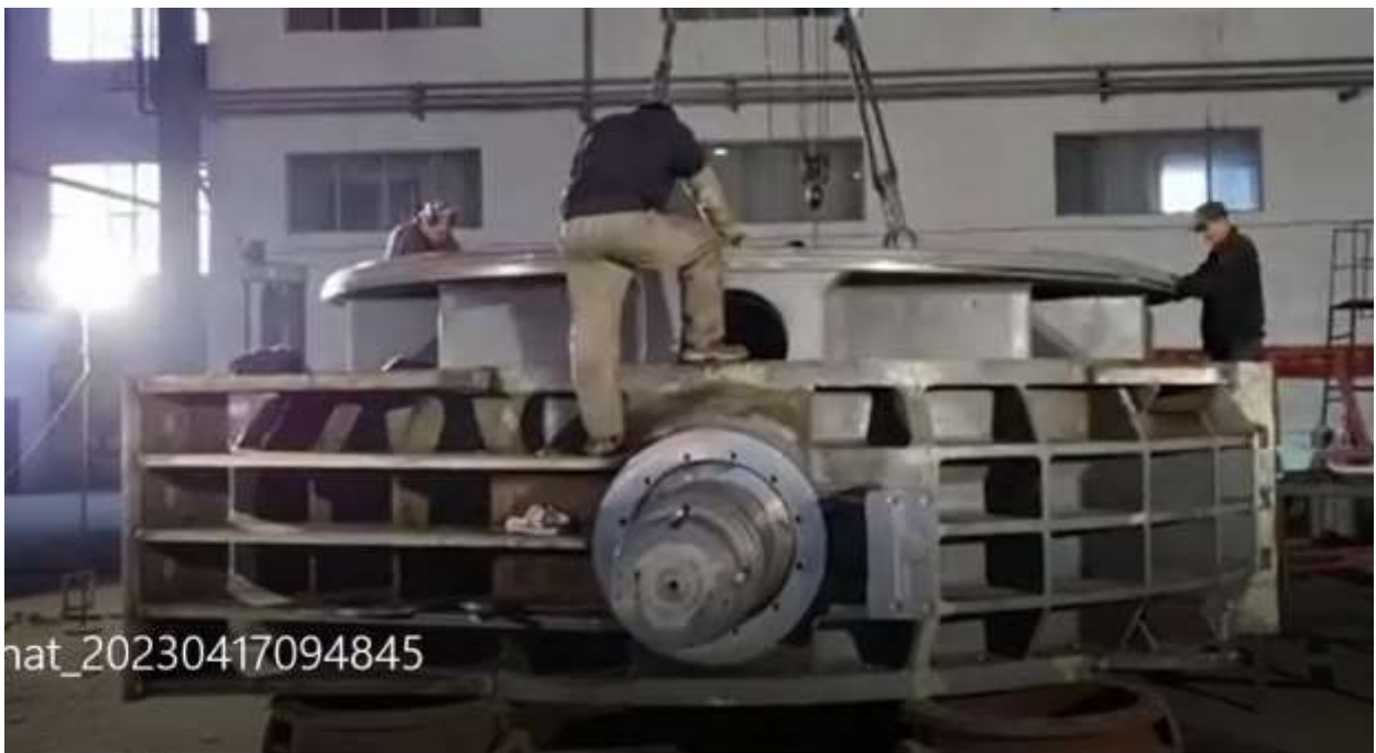
Figure 2-37: PPV disc being assembled with PPV body
